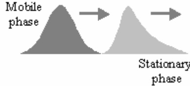
Figure 3. Distribution profiles for an ideal (left) versus a non-ideal (right) chromatographic column.
