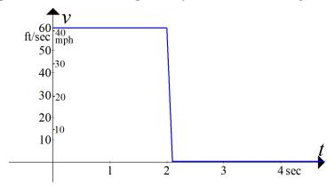
The velocity v(t) = s'(t) is the derivative of s(t), the distance driven or odometer reading, so the *level* of the velocity graph is the *slope* of the distance graph. Thus s(t)has constant slope 60 ft/sec until t = 2, then suddenly zero slope: the car has stopped.
