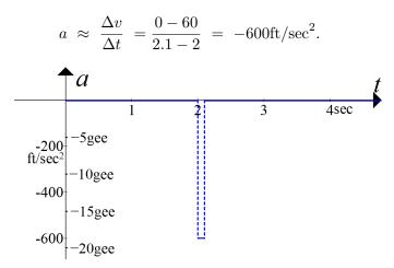
What physical story do these graphs tell? The car went from about 40 mph to zero in 0.1 sec. Brakes cannot decelerate so quickly: this is a car crash. The deceleration graph is zero for most of the time, but for a split second it is almost 20 gees, twenty times your weight pressing you into the seatbelt.
